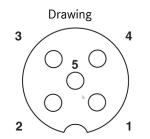
Pin assignment M12-jack, 5 pol, A-coding
