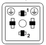
Pin assignment valve plug, design CI
