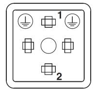
Pin assignment valve plug, design CI
