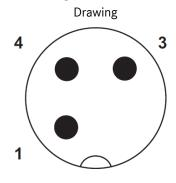
Pin assignment M12-plug, 3 pol, A-coding
