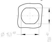
Tin cut-out for torsional protection
