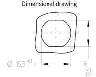
Tin cut-out for torsional protection
