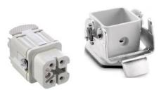
H-A 4 Female Screw termination 4 + PE 1 mm Screw termination: 0,5 - 2,5 mm<sup>2</sup> (2,5 mm<sup>2</sup> with wire end sleeve, depending on crimp profile) IP 65 (latched) 12, 4 (latched) 100 -40°C to +125°C, short term up to +125
