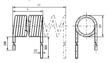
Unextended spiral length max, extended length of spiral Approx. outer diameter of spiral Approx. outer diameter of cable
