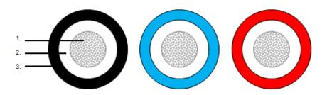
1. Conductor: Fine wire strands of non-porous tinned copper wires acc. to IEC 60228 resp. EN
